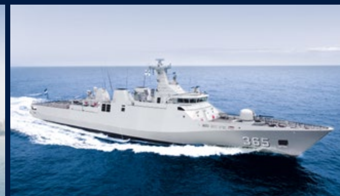
SIGMA Class Corvette of the Indonesian Navy with two 10 MW CODELAG diesel propulsion drives and each 1,3 MW electric motor
