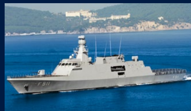
Turkish Navy MILGEM class corvettes with a 30 MW CODAG cross connect propulsion train onboard, including one gas turbine and two diesel engines.
