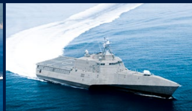
Austal's Independence class Littoral Combat Ship (LCS) of the United States Navy with four separate waterjet drive trains, two gas turbines and two diesel engines, 65 MW total power.
