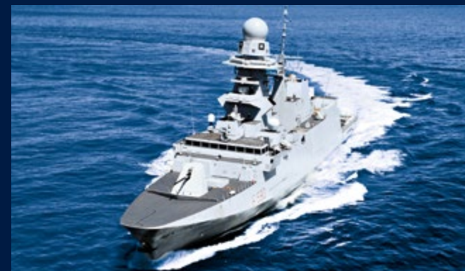
Italian Navy Carlos Bergamini class frigates with a 36 MW CODELAG propulsion plant onboard, featuring one gas turbine and the two electric motors on the propeller shafts. Gears produced in cooperation between RENK and Fincantieri.
