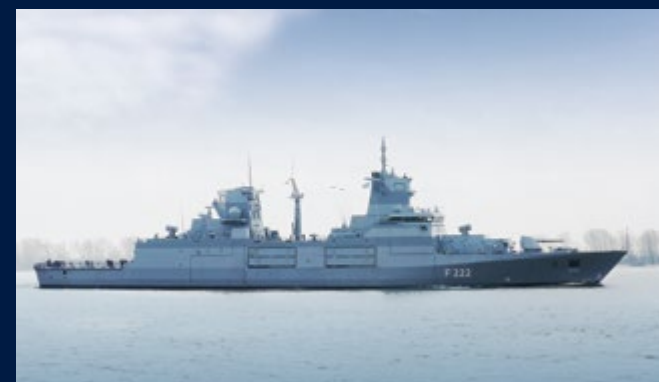
German Navy Baden-Württemberg class frigates with a 29 MW CODELAG cross connect arrangement including one gas turbine and the two electric motors in front of the gears
