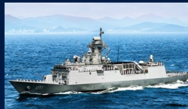
South Korean Incheon class frigates with 2x24 MW traditional CODOG onboard, including two gas turbines and two diesel engines.
